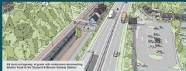
A9 dual carriageway at grade with underpass reconnecting Station Road to the Dunkeld & Birnam Railway Station
