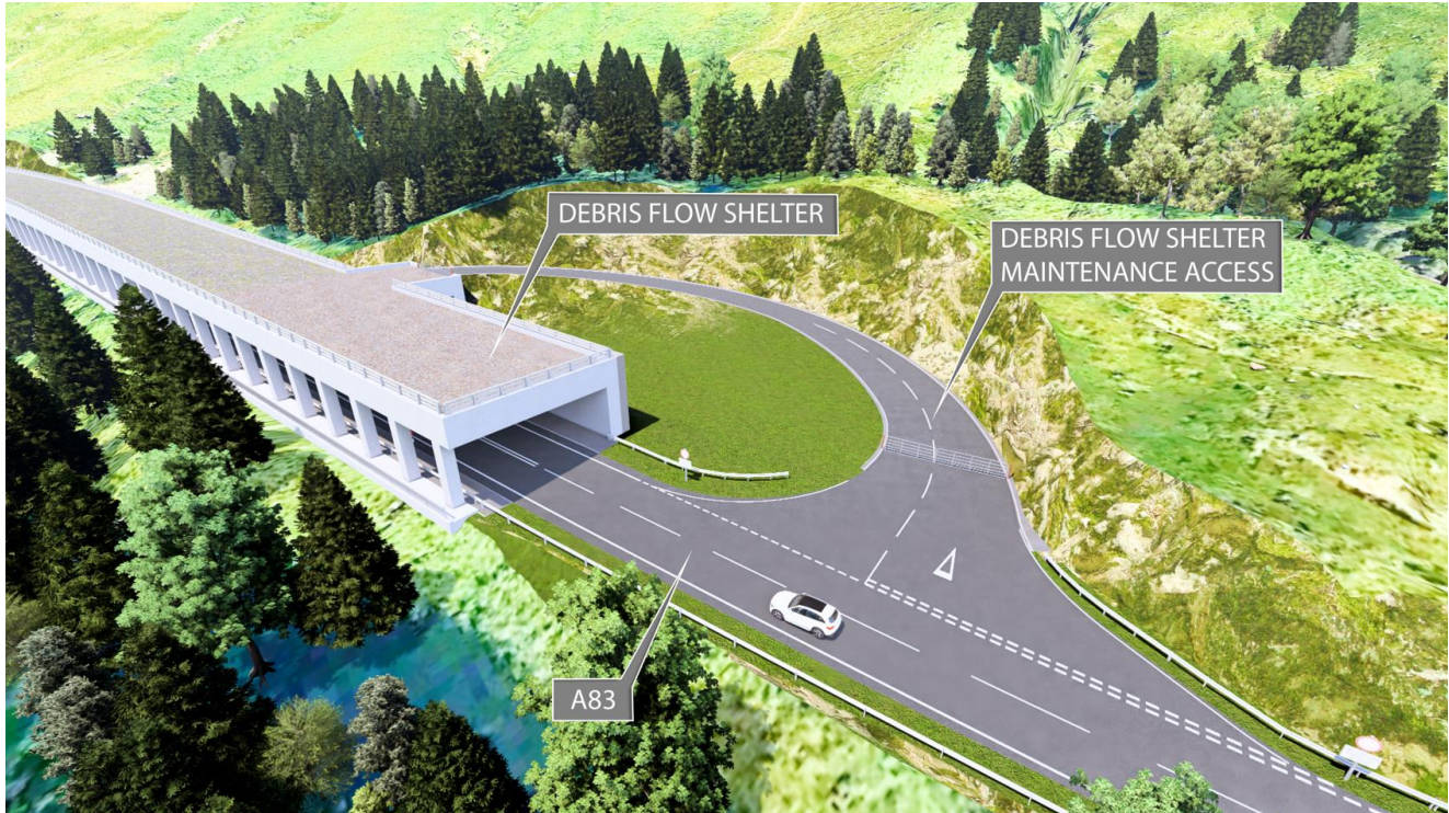
Figure 1-3 – Debris Flow Shelter and associated maintenance access (Visualisation)
