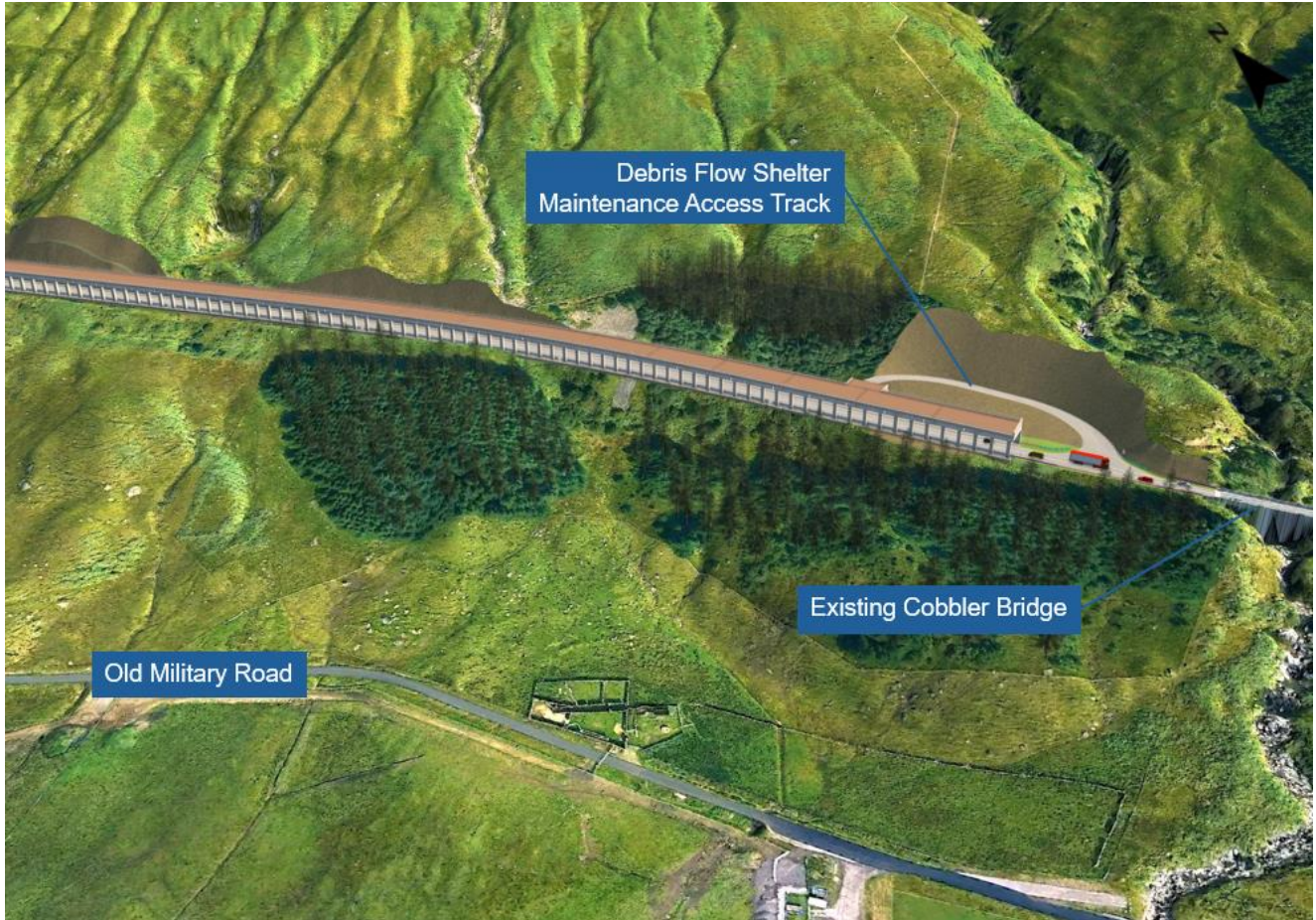
Figure 3-7 – Computer generated image of the DFS at the southern end of the Proposed Scheme
