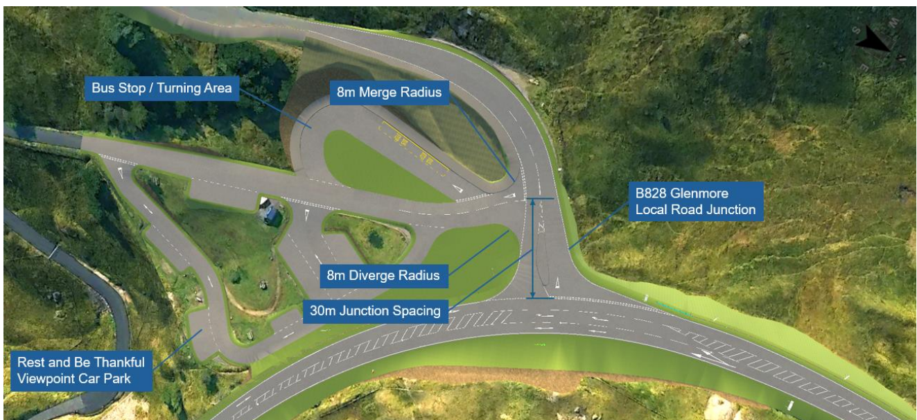
Figure 4-3 – Rest and Be Thankful Viewpoint car park junction with pertinent features labelled
