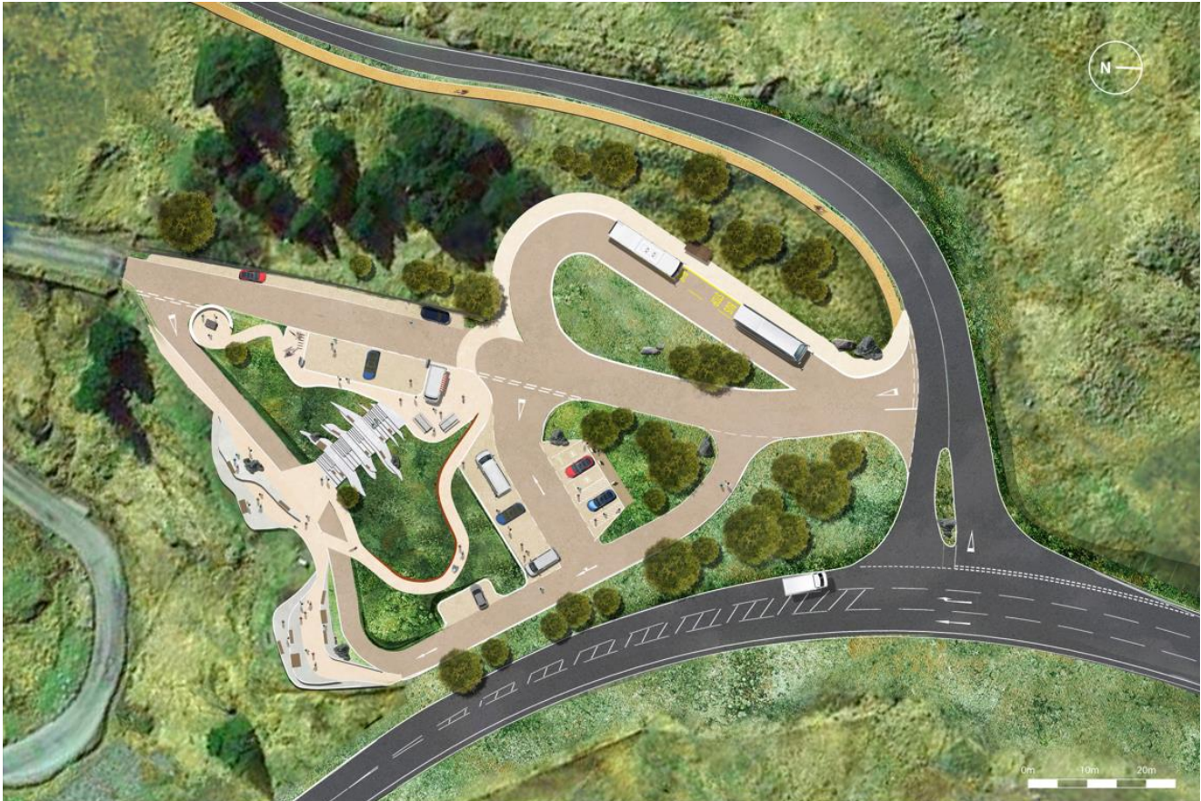
Figure 3-3 – Concept design of the proposed Rest and Be Thankful Viewpoint car park improvements with a single junction providing access to the car park and an integrated bus stop / turning area
