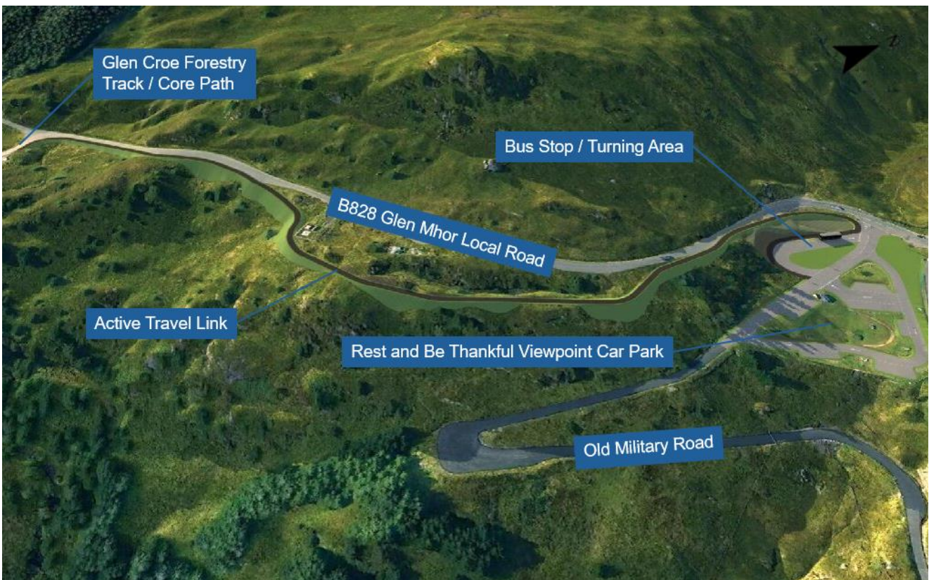
Figure 3-4 – Plan view of the proposed Active Travel Link adjacent to the B828 Glenmore local road connecting the Rest and Be Thankful Viewpoint car park to the Glen Croe Forestry Track / Core Path
