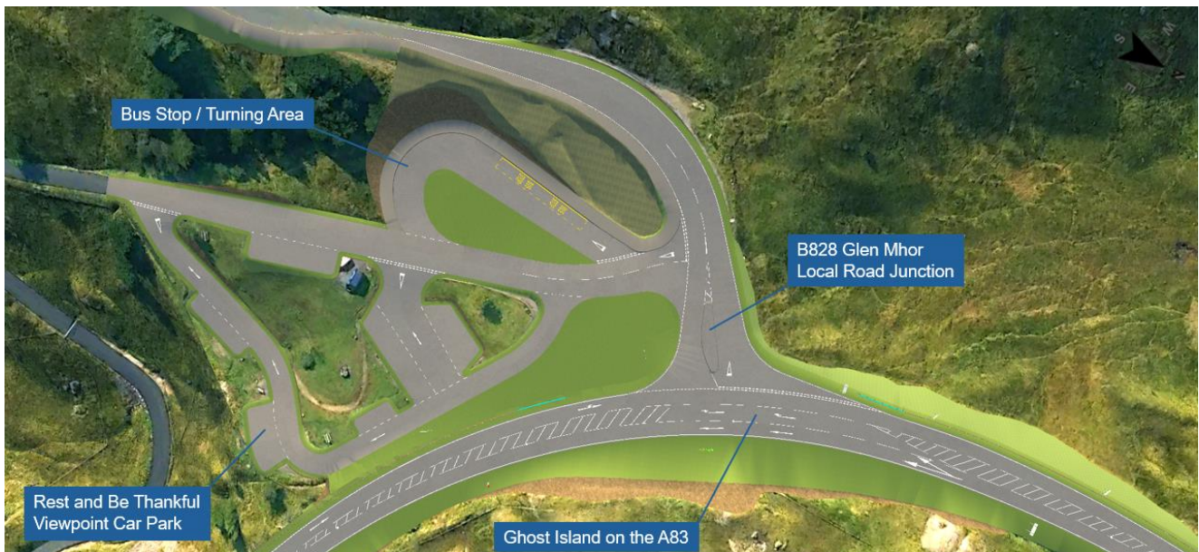
Figure 3-1 – Plan view of the proposed junction between the A83 and B828 Glenmore local road including the ghost island on the A83 and the channelising island on the B828
