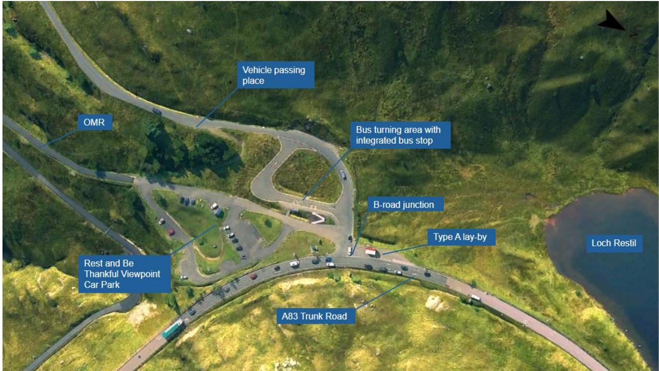
Figure 2-1 – Plan view showing the existing A83 / B828 Glenmore local road junction including the Rest and Be Thankful Viewpoint Car Park and Bus Stop / Turning Area
