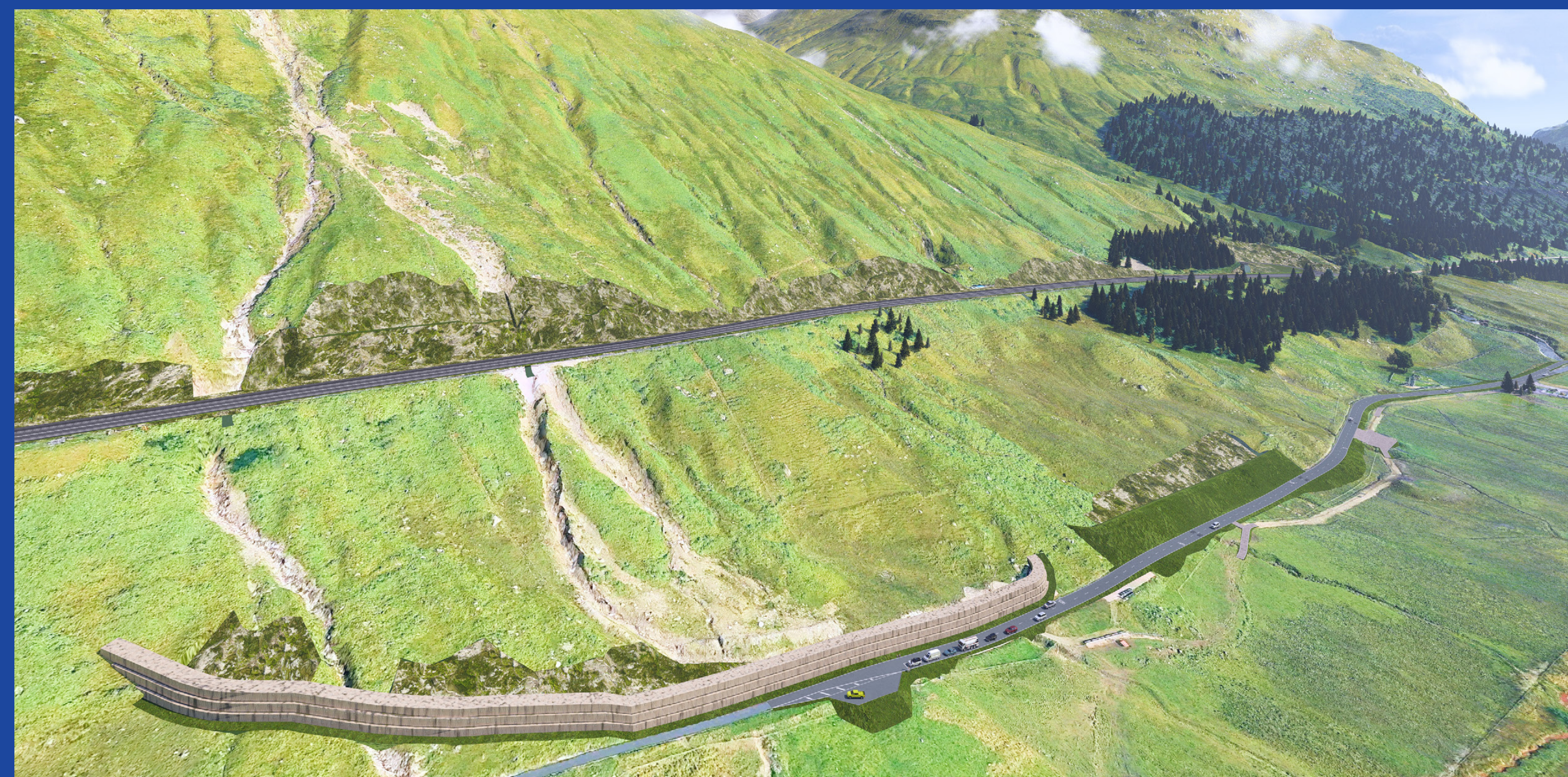
Visualisation of OMR interventions, including the extension of two-way widening, earthworks bund and the extension of the HESCO barrier
