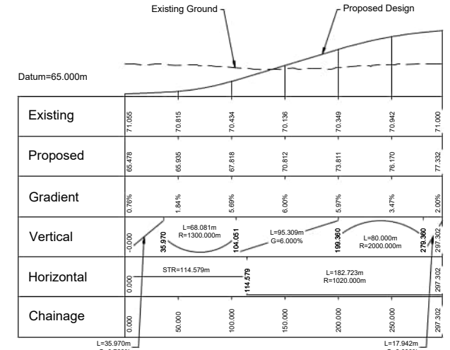
Murthly Junction Northbound Merge (Design Speed 60kph)
