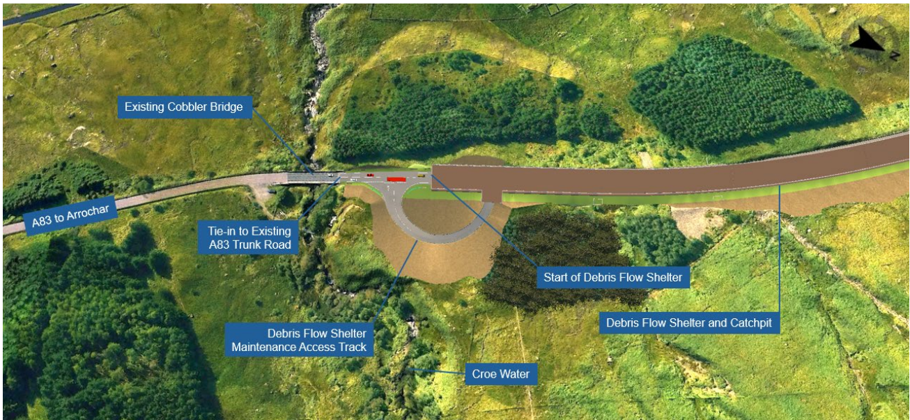
Plate 4.4 – Plan view of the proposed direct access and maintenance track located immediately north of the Croe Water (Cobbler Bridge) providing maintenance access directly to the roof of the DFS
